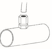
**Step 3:** Now connect the delivery tubing to the Pipe Injector, turning the compression nut clockwise until hand tight.
